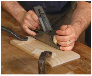
Install the panel. On drawer bottoms, only one end needs to be beveled since there's no groove in the drawer back. Instead, the bottom extends over the narrow back and is nailed to it.
