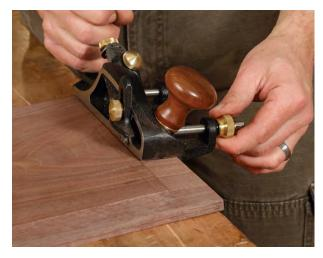
Tilt the plane to bevel the ends until they fit in the groove. Guess the correct angle at first, then check your progress by eye and feel after several passes. Adjust the plane's angle as necessary and continue. Eventually the plane will register itself, right or wrong, so check your work regularly.
