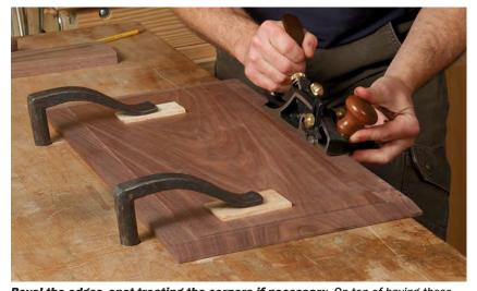
Bevel the edges, spot-treating the corners if necessary. On top of having these bevels be consistent and smooth, you want them to intersect with the cross-grain bevels and produce a nice, clean, straight line from the corner of the raised field to the corner of the panel.
