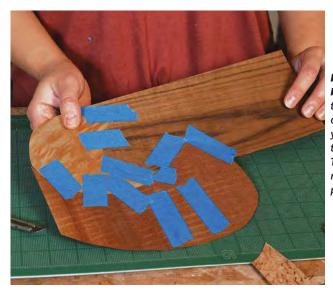
Reinforce the back. Remember to tape the back of the panel as you work through the process. This tape will be removed later prior to glue-up.
