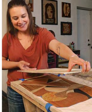
Glue the veneer to a backing. Apply a thin layer of glue to the substrate, using a scrap piece of veneer as a spreader. The glue should be spread thin enough that it doesn't run when held vertically. Place the substrate down on the veneer and secure it with tape.
