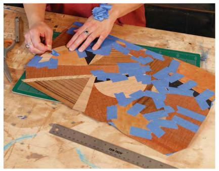
Remove tape from the back. Carefully remove tape from the entire back of the panel, as this will be your glue surface. If a small break develops or a piece of veneer begins to lift, simply press it back into place.
