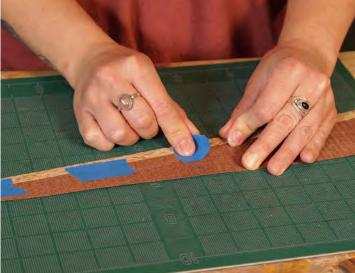
Joining straight edges. As before, use a metal ruler for cutting straight lines accurately, taking multiple light passes when going with the grain. Pinch narrow pieces together before applying tape to create a tight seam. Don't be afraid to stretch tape across multiple pieces.
