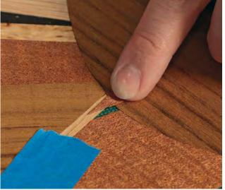
**Making small** repairs. If a small piece of veneer breaks off, put some blue tape on the back, then press the small piece back into place.
