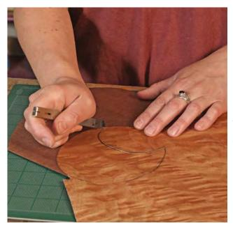
Make the next cut. Working from the front again, go on to the next cut. As ever, be sure to hold your knife perpendicular to the veneer.
