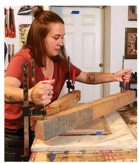
**Clamp with what you have.** A vacuum veneer press does a good job, but a combination of clamping cauls and plywood also works well to distribute even pressure across the panel. Using a corner of your bench allows you to apply the maximum amount of clamps. Once glue is dry, sand with 120-grit, 220-grit, then a gray Scotch-Brite pad. The finer grits can be hand-sanded in areas where crossing grain is an issue.
