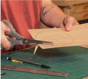
**Cutting straight** lines and curves. Using a metal ruler and a knife with a snap blade, Van Voorhis uses a few light passes to make a clean, straight cut. A pair of scissors makes easy work of cutting curves or cutting through grain that would be more difficult with a knife.
