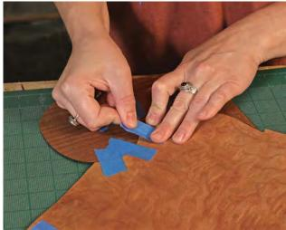
veneer with tighter grain. I am also mindful of grain direction when laying out a panel. Placing two pieces next to each other with alternating grain gives the panel contrast and chatoyance.
