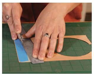
Cutting short grain. Applying blue tape to the veneer when cutting across the grain prevents splitting.
