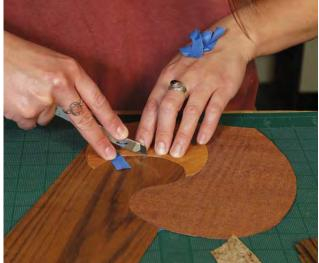
Build the pattern as you go. With the first two pieces joined, you can add a third. Tape in multiple places to help hold veneer for accurate cutting.
